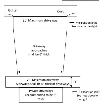
1/2" expansion joints shall be used at these two locations and shall completely separate all concrete in the driveway approach and driveway from the concrete in the sidewalk and in the curb, including the rolled-up portion of the curb and driveway approach.
