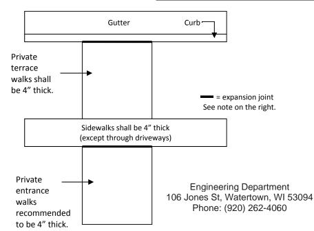
1/2" expansion joints shall be used at these two locations and shall completely separate all concrete in the terrace walks from the concrete in the curb and shall completely separate all concrete in the entrance walk from the concrete in the sidewalk.
